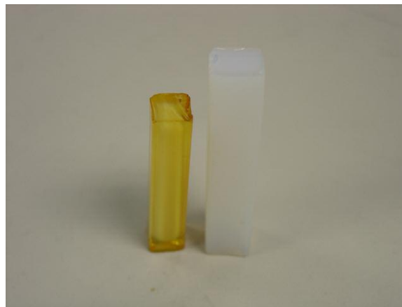
Figure 6 Sample shrinkage and change in surface morphology of CSA sample at - 180C
